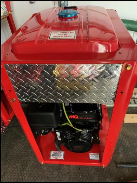
The Hydro-Halo wildfire prevention system is equipped with 2 fuel tanks and 3 shut-off valves. **When not in use all three valves should be in the OFF position.**
