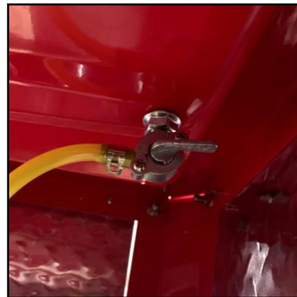
Placed on the top of the main tank is the sticker stating "**FUEL SHUT-OFF UNDER TANK**". Located directly under this sticker is the **Main Tank Fuel Valve**, one of the three fuel valves. Above right picture showing valve in the "**Off Position**". (Handle to horizontal right position.)
