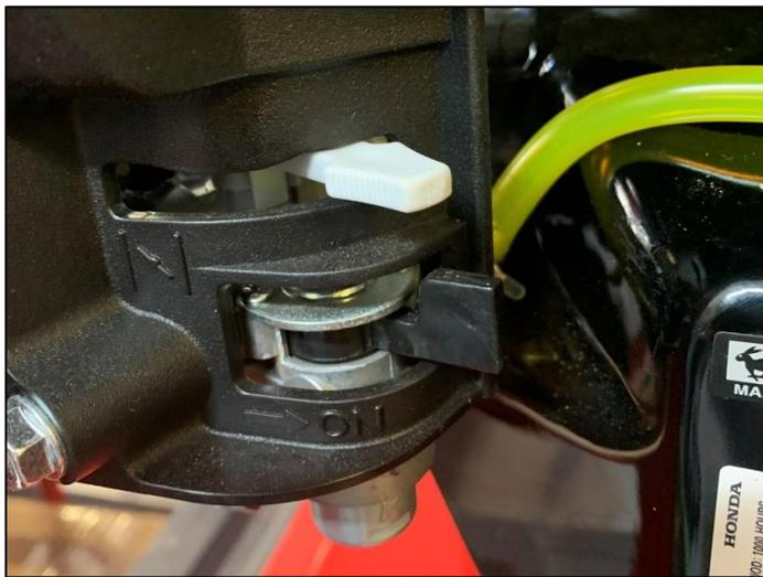
Pictured left is the factory Choke lever (White) and Fuel Lever (Black).
